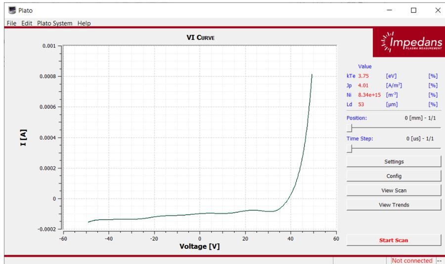
Figure 1: Typical IV characteristic of Plato probe.
